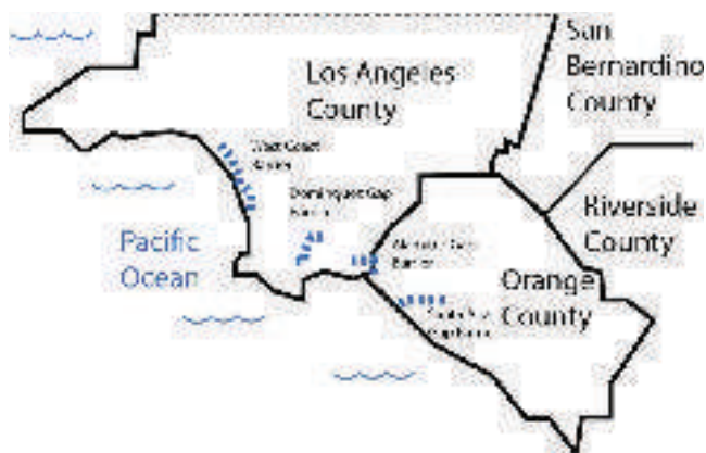
FIGURE 2-4 Locations of the four major Southern California seawater barriers employing reclaimed water. These barriers range in length from 2 miles (Alamitos Gap) to 9 miles (West Coast Barrier).
